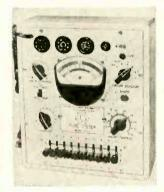
voltage regulator, miniature votage regulator, miniature tubes, etc. Free-point selector system circuitry. Double fuse protection for meter and transformer. Loose-leaf book with tab-indexed tube chart cards allows for insertion of additional cards. Illustrated detailed instructions for building it instructions for building-it-yourself.— General Electronic Equipment Co., Mantua and Glendale Sts., Easton, Pa.
